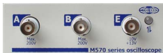
Fig. 3.1.1.1. – Front panel of the M570 series oscilloscope
