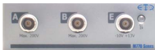
Fig. 3.1.1.3. – Front panel of the M770 series oscilloscope
