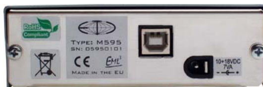
Fig. 3.1.3.1. – M595 rear panel layout
