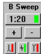
to be displayed on the oscilloscope screen. Default setting is 400 samples from 8000. This is indicated in the upper part of the B Sweep window by 1:20 label, because just 1/20 of stored samples is displayed. By clicking the “+” or “-” buttons it is possible to change the display ratio from 1:2 to 1:20 (See tab. 3.2.10)
